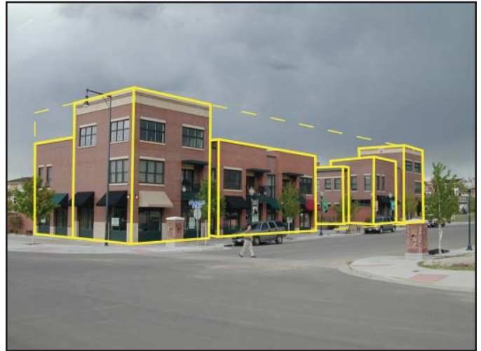
Proportion is the relationship, size and shape of one part of a form or space to another part of a form or space. In this photo, the proportion of the building breaks the mass into smaller components.
