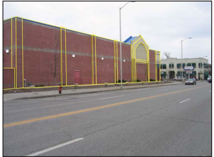
This building displays good building orientation in that it helps to define the street edge and good proportions in that the mass is broken up into a rhythm of smaller scale elements. However, this building lacks proper directional relationship and articulation .
