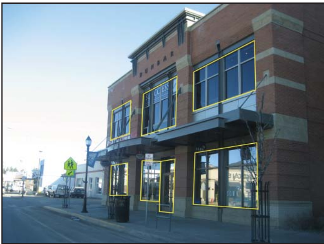
Permeability refers to the ease of interaction between the interior of the site or buildings and the streetscape or other civic spaces on the exterior. This building displays good permeability to the streetscape, which invites customers to view items for sale within the building.
